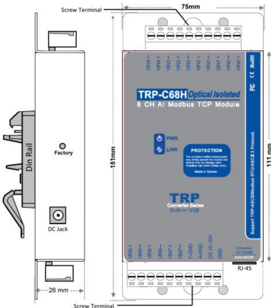
**Notice:** The Module provides two type power inputs, optional DC-JACK or Screw Terminal input, not to two used together!
