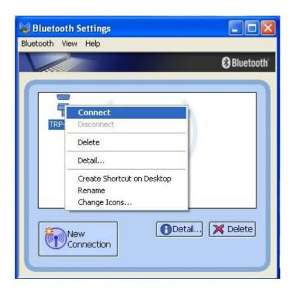
Select "Connect" option you are requested a Bluetooth passkey. Please Input TRP-C51 password which must be same as the setting by TRP-BT utility, press OK, TRP-C51 will go into searching mode, the LINK LED start to fast blinking.
