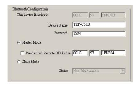
In TRP-C51 paired mode, it is necessary to set same name and password for both TRP-C51 (Master and Slave) .
