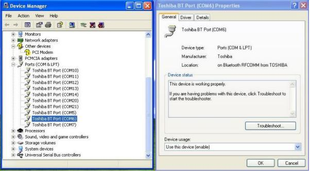
User may back to the Windows screen and Click Start – Program file – Bluetooth – Bluetooth setting to start the second TRP-C51 installation. The number of TRP-C51 that a Host system may install is depended on the COM Port number that the system or OS can offer.
