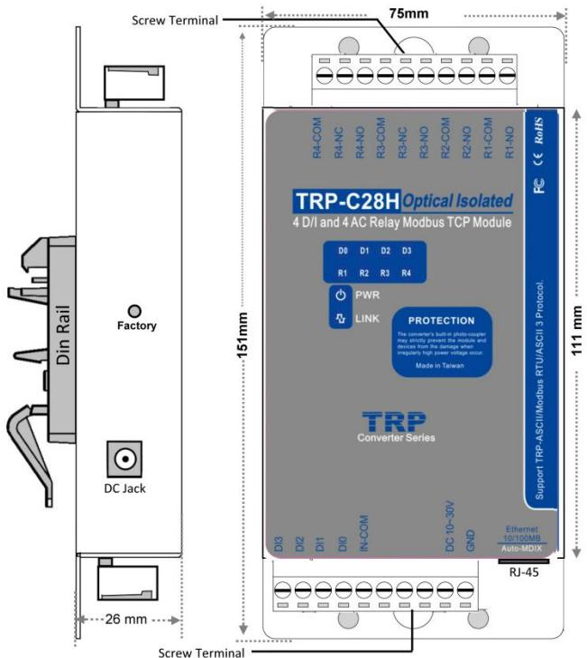
**Notice:** The Module provides two type power inputs, optional DC-JACK or Screw Terminal input, not to two used together!
