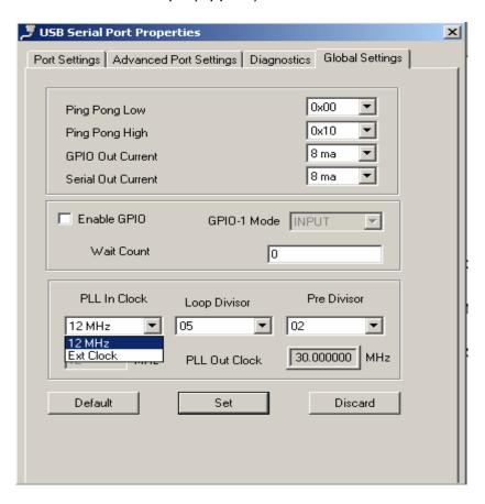
Custom baud rates can be derived under PLL Out mode through External Clock option also. Either using Table 1 values of DLL, DLM or by Enabling DLL/DLM. M, N values and Clock source value (Frequency) determine Input Frequency.
