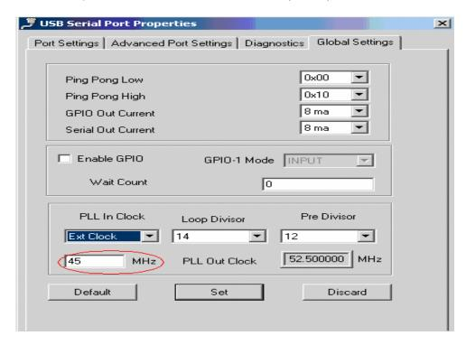
"PLL In Clock" can be either 12MHz from crystal or External Clock Source. When "Ext Clock" is selected, user needs to enter the external clock frequency in the box shown above (Red Color) to get the desired output clock from PLL.
