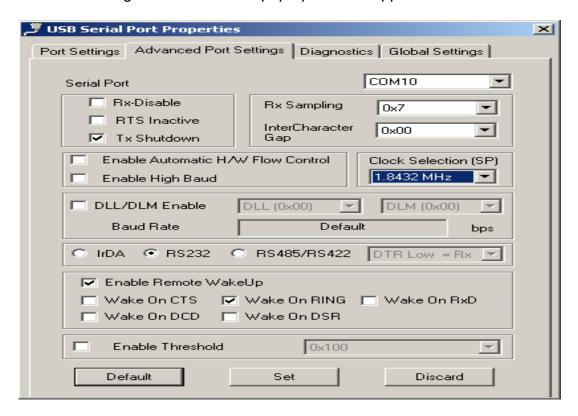
For baud rate support upto 921600 bps "Enable High Baud" option to be left unchecked. For baud rates above 921600 bps this box to be checked for respective serial port.
