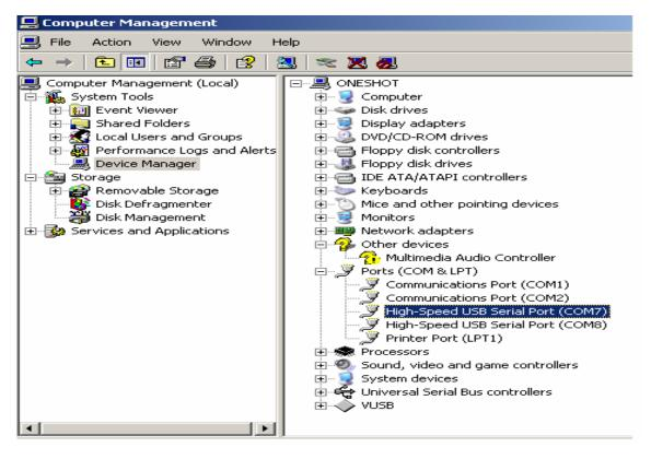
Right Click on High-Speed USB Serial Port(COMX) > Properties > Features. A new window will pop up as shown below. Under normal default operation, driver will ignore the advanced baud rate settings. The driver will set the divisor values as such a 1.8432 MHz crystal is present.
