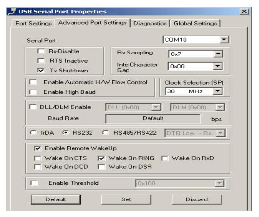
If Clock Selection = 30MHz and baud rate selected is 9600baud in terminal application, then the actual set baud will be calculated as below.
