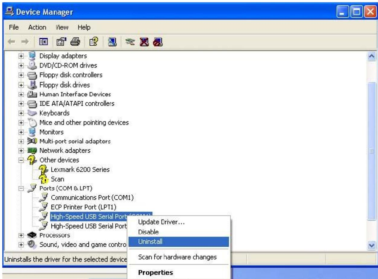
The OS will prompt the user whether to uninstall the device from the system. Click on “OK” to uninstall or “Cancel” to terminate the un-installation.
