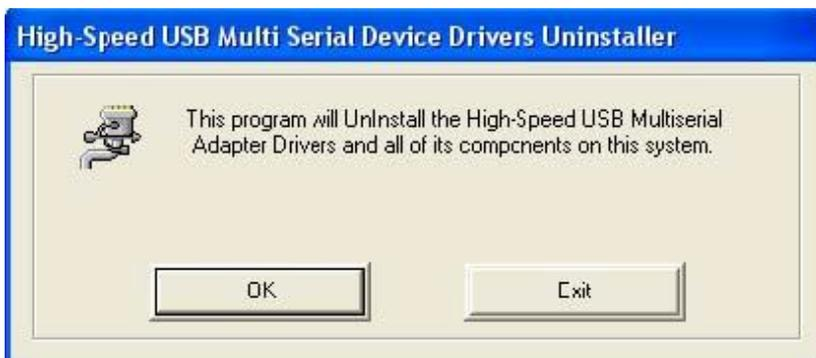
Use the “**Exit**” button to complete the Uninstaller utility. No need to restart the PC, unless prompted by the OS. The driver can also be uninstalled from **Control panel – Add / Remove Programs**. Select the “High-Speed Multi Serial Compound Device” from the Add / Remove panel and click on “**Remove**” option. This will remove the MCSTRP-C08H device driver from the PC.
