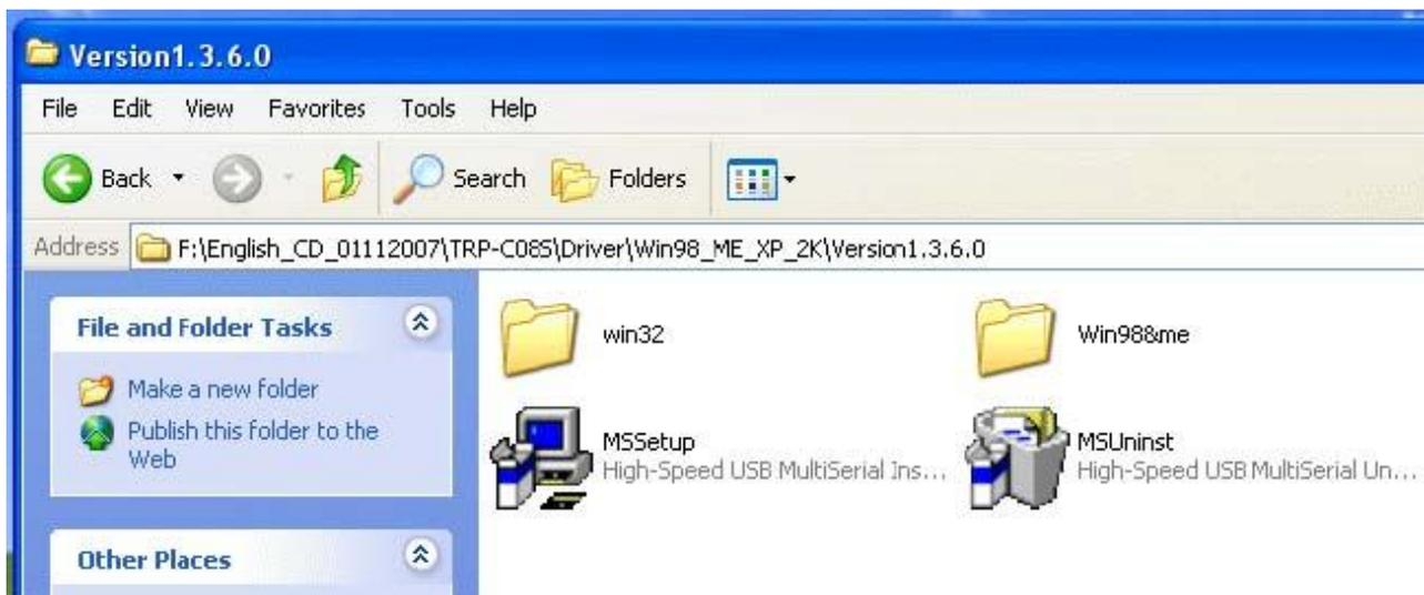
Use "MSSetup.exe" utility to install the driver. Double click on the utility to start the installation process. Press "Install" button to install the drivers for High-Speed USB Multi serial Device.
