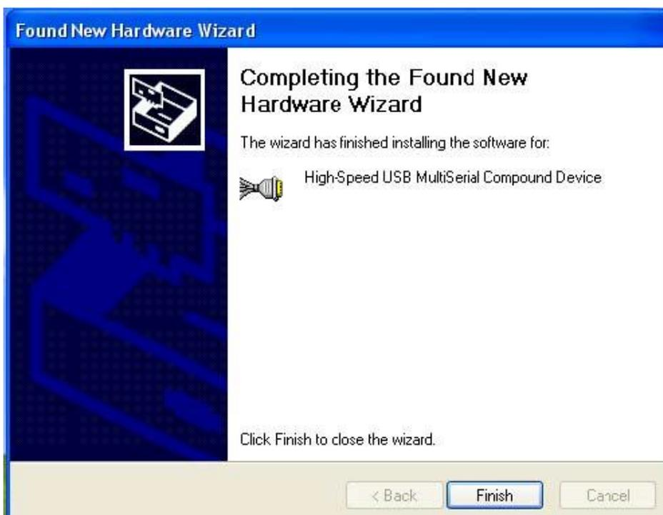
TRP-C08H device detection can be confirmed by checking the Device manager. Check for “High-Speed USB Multi Serial Compound Device” under Universal Serial Bus Controllers and “High-Speed USB Serial Port (Com X)” under the category Ports (COM & LPT)
