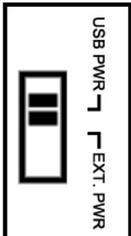
1. Find the power select switch which is located at the right side of USB port.
