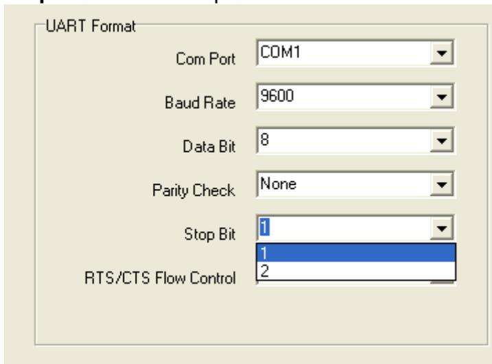
The screenshot shows a 'UART Format' dialog box with the following settings: Com Port: COM1, Baud Rate: 9600, Data Bit: 8, Parity Check: None, Stop Bit: 1, and RTS/CTS Flow Control: 2. The 'Stop Bit' dropdown menu is open, showing '1' selected and '2' as an alternative option.
