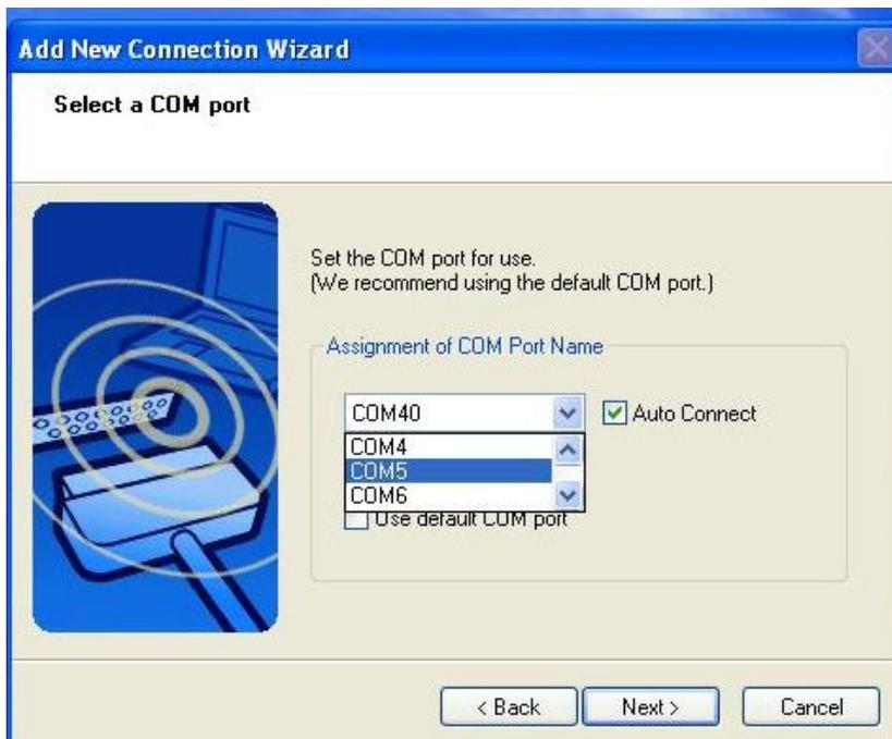
“Auto Connect” means TRP-C51 will automatically connect when encounters unexpected disconnection.” User may choose the function enable or disable.
