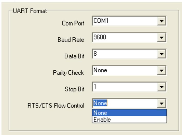
The screenshot shows the 'UART Format' dialog box with the following settings: Com Port: COM1, Baud Rate: 9600, Data Bit: 8, Parity Check: None, Stop Bit: 1, and RTS/CTS Flow Control: None. The 'RTS/CTS Flow Control' dropdown menu is open, showing 'None' selected and 'Enable' as an alternative option.
