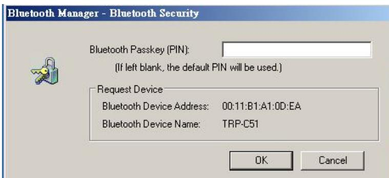
**Step9:** When TRP-C51 is successfully connected user may see the next screen, the LINK LED stop fast blinking and turn to lighting. TRP-C51 is available to data communication or control. You also may find TRP-C51 has already been added in system device manager.
