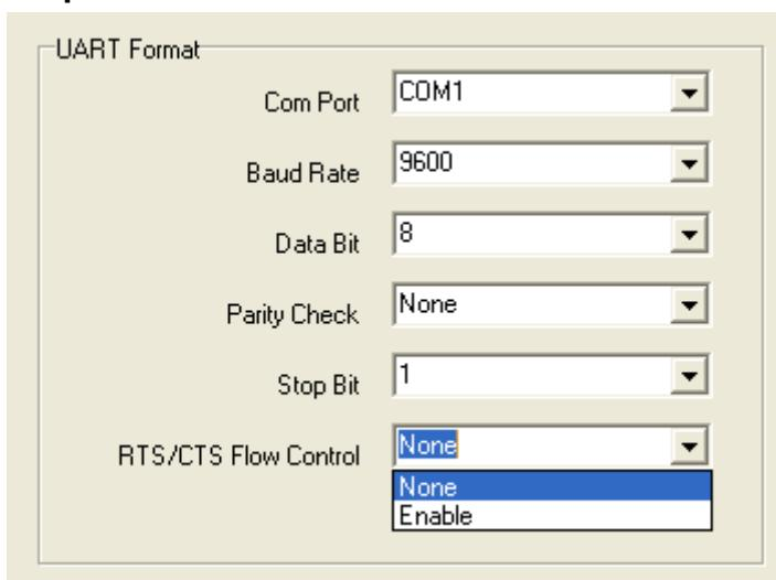
**\*It must be set to NONE when RS422/485 operation.**
