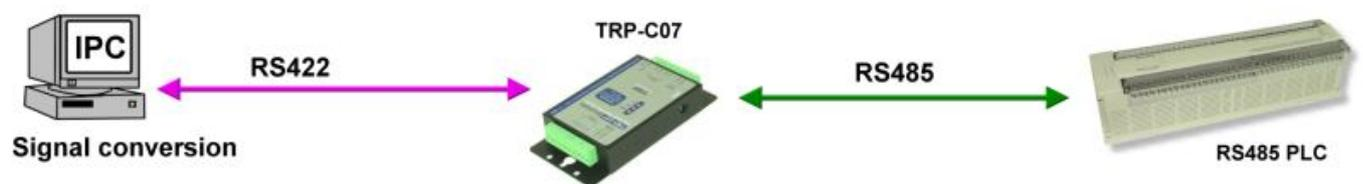
\*TRP-C07 support bi-directionally communicate between RS422 and RS485 devices
